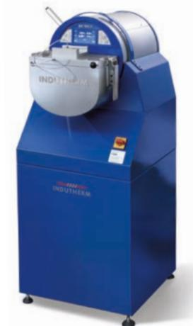
The MC 100 V as a stand-alone version: The floor stand provides enough space for accessories such as the vacuum pump.
