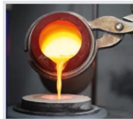
*Melting by induction technology: The crucible containing the material is placed in the core of the induction coil. A strong alternating magnetic field generates a strong alternating current in the graphite crucible and in the metal. This results in rapid heating and thorough mixing of the material.*
