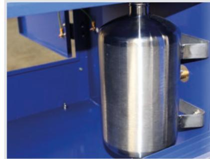
An additional pressure tank integrated into the plant provides for even faster pressure build-up for activation of the Turbo Pressure PLUS function.
